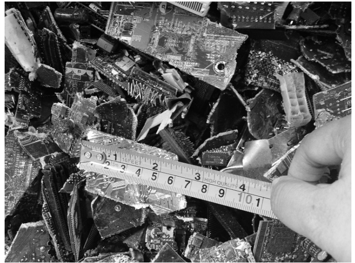
Chips particle sizing - output from a Quad®
